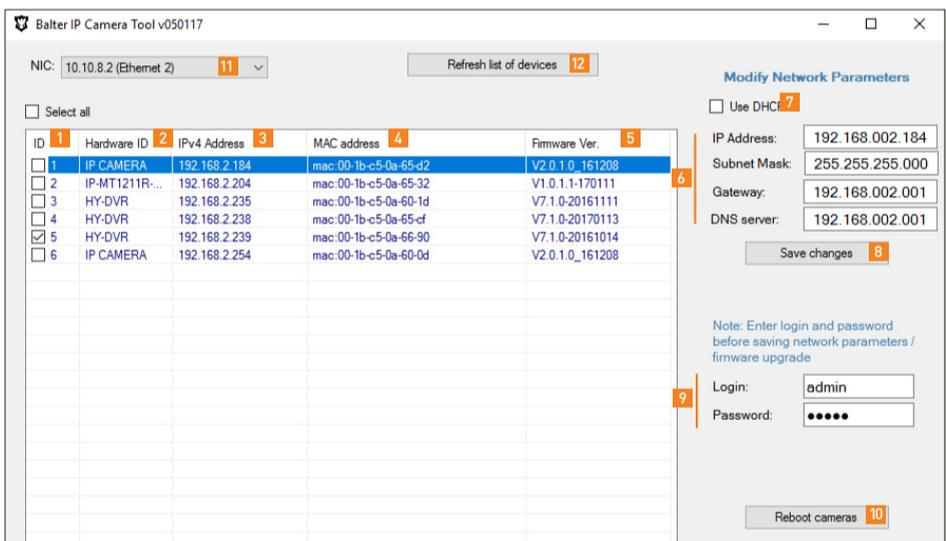
1. ID Number | 2. Device Type | 3. IP Address | 4. MAC Address | 5. Firmware Version | 6. Network Configurations - Input Fields for IP Address, Subnet Mask, Gateway, DNS Server | 7. Enable DHCP (Currently not available) | 8. Save Changes | 9. Login Data - Login und Password Input | 10. Reboot Cameras | 11. Network Card | 12. Search
