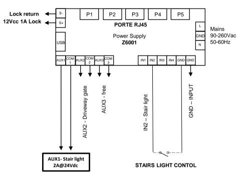
WIRING DIAGRAM DOOR RELESE CONTROL
