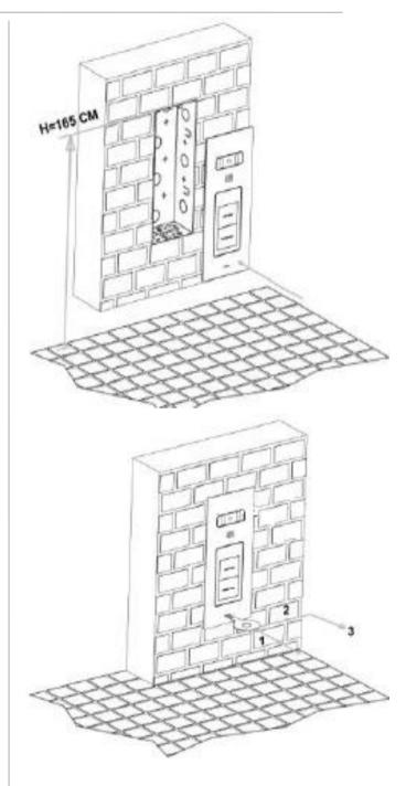
To remove the Entrance Panel use the appropriate extraction key.
