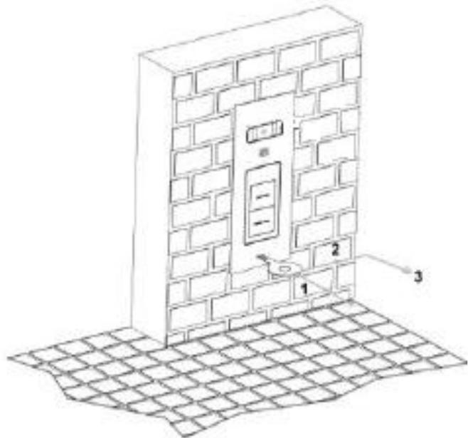
To remove the Entrance Panel use the appropriate extraction key.
