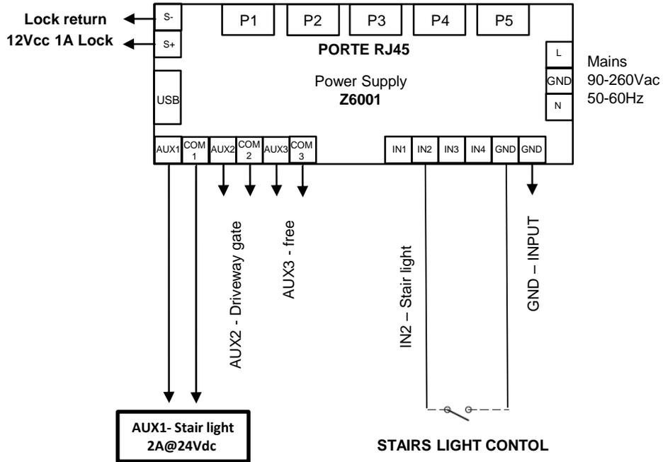
WIRING DIAGRAM DOOR RELEASE CONTROL
