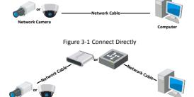
Figure 3-2 Connect via a Switch or a Router
