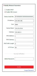
Figure 3-5 Modify the IP Address
