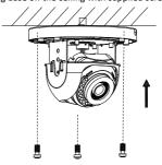
Figure 2-3 Fix the Mounting Base
