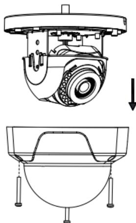
Figure 2-2 Remove the Bubble
