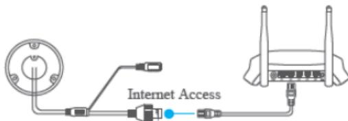
Figure 5-3 Connect a Router
