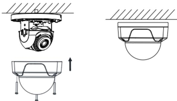
Figure 2-6 Bubble Reinstallation
