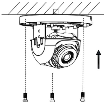
Figure 2-3 Fix the Mounting Base
