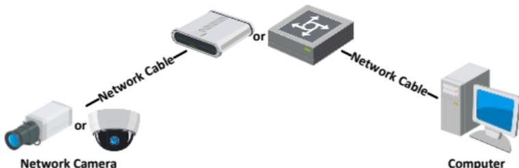
Figure 3-2 Connect via a Switch or a Router
