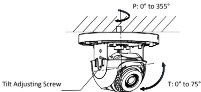
Figure 2-5 Type I Camera 2-Axis Adjustment
