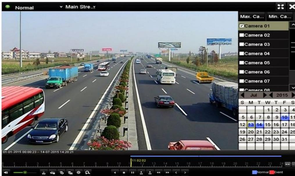
Figure 6-9 Interface of Playback by Time
