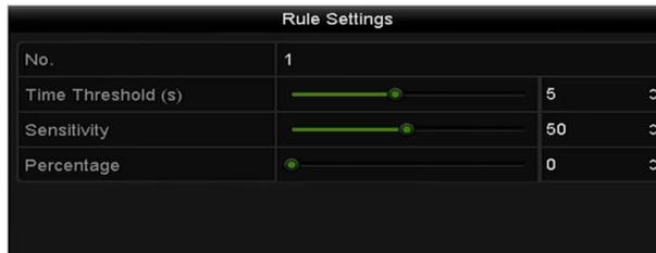
Figure 9-7 Set Intrusion Crossing Detection Rules
