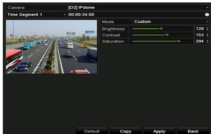
Figure 13-6 Image Settings Interface (IP Camera)
