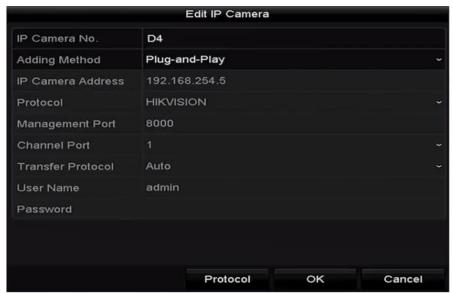
Figure 2-37 Edit IP Camera Interface - Plug-and-Play
