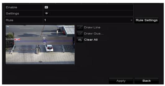
Figure 9-4 Draw Line for Line Crossing Detection
