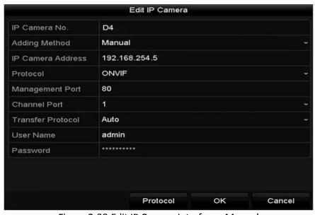
Figure 2-38 Edit IP Camera Interface - Manual
