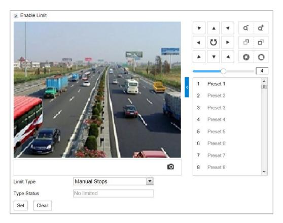
Figure 5-23 Configure the PTZ Limit
