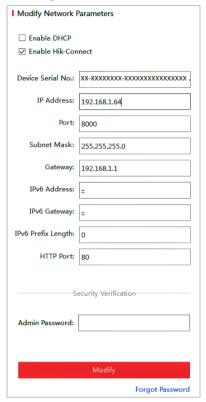
Figure 2-5 Modify the IP Address
